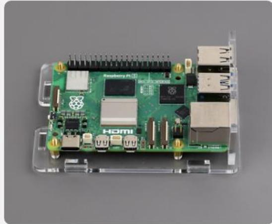
2. Install the 5th acrylic panel to the USB ports and Ethernet port of Raspberry Pi 5, and then mount Raspberry Pi 5 on the short standoffs as shown.
