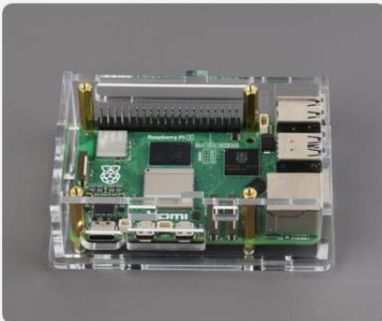
3. Fix the Raspberry Pi 5 via long standoffs, then install the 3rd, 4th, and 6th acrylic panels.
