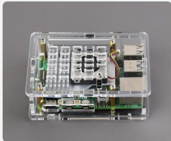
4. Install the active cooler on the Raspberry Pi 5, then install the 2nd acrylic panel on the top and fix it via screws.
