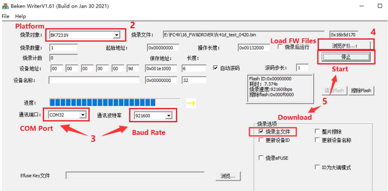
Figure 15: Configurations for Firmware Upgrade
