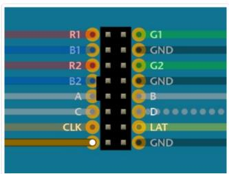
**OE** connects to Arduino pin **9**. This is the same for both the **Arduino Uno** and **Mega**.
