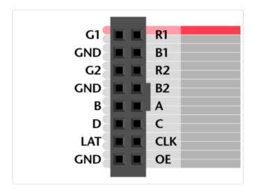
**Either end of the ribbon cable can be plugged into the matrix INPUT socket.** Notice below, the "key" faces the same way regardless.
