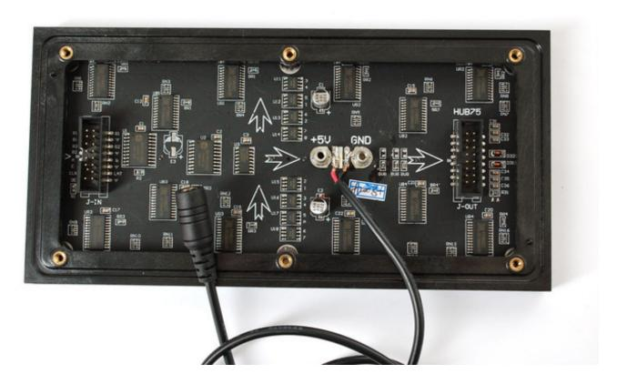
If your panel has the Molex-style header, just plug in the included power cable, observing the correct polarity.
