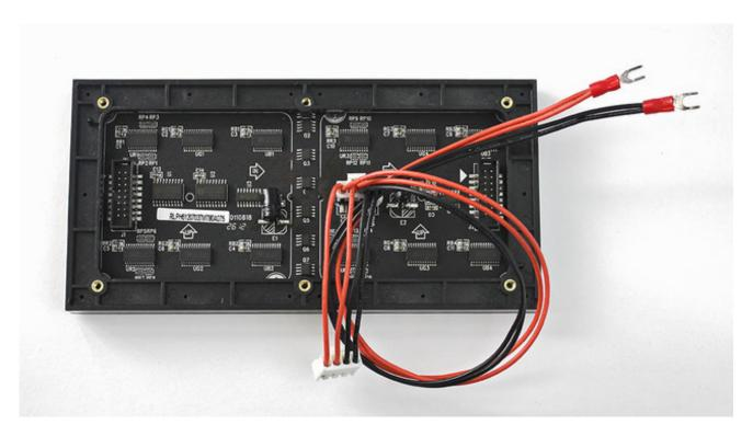
The spades at the opposite end of this power cable can be screwed into a 2.1mm terminal block adapter. Works nicely! Don't allow the exposed connectors to contact metal though...you should
