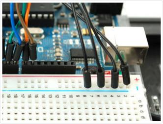
Current **Arduino Uno** boards have **three** ground pins (the third is next to pin 13). If you need additional ground connections — for a 32x16 matrix, or if using an older Arduino board with only 2 ground pins — a solderless breadboard is handy for linking all these pins.
