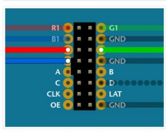
Pins **R2**, **G2** and **B2** (labeled R1, G1 and B1 on some matrices) deliver data to the **bottom half** of the display. These connect to the next three Arduino pins...
