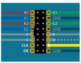
For **32x32** and **64x32** matrices, **LAT** connects to Arduino pin **10**.
