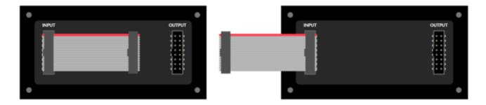
A dual-row header gets installed on the proto shield, similar to the connector on the matrix. Just like the ribbon cable lying flat, as long as these two headers are *aligned the same way*, they'll **match pin-for-pin**; unlike the jumper wire method from the prior page, mirroring doesn't happen.
