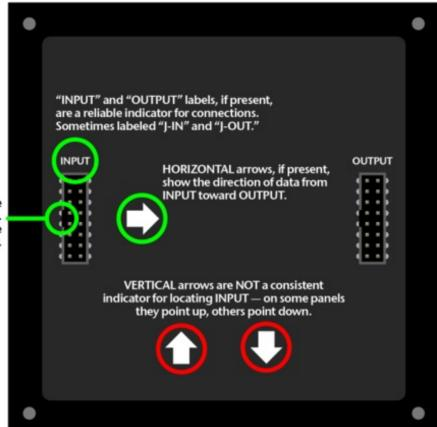
If there are no labels of any kind, the notch in the header shroud is a hint. On the INPUT connector, it faces the outer edge of the panel, not the center. The arrangement of pins on the INPUT connector varies with matrix size and the batch in which it was produced...
