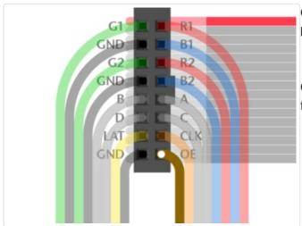
**OE** connects to Arduino pin **9**. This is the same for both the **Arduino Uno** and **Mega**.
