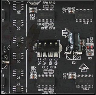
On the left is a screw post power connector (with adjacent pads for soldering wires directly). On the right, a Molex-style header. Some panels will have *two* headers...the power cable included with these panels has connectors for both headers.
